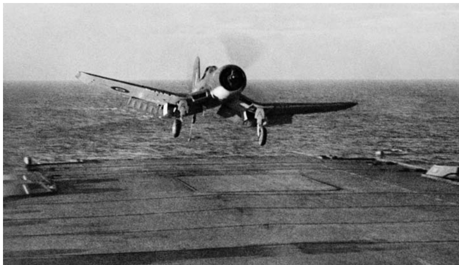
ABOVE: An F4U Corsair comes in for a landing aboard an aircraft carrier in the Pacific. Although its early trials as a carrier-based fighter revealed some problems, the Corsair was eventually adapted to operations aboard carriers and proved to be a fine dogfighter and ground-support aircraft. OPPOSITE: The Chance Vought F4U-2 Corsair made its combat debut in the Pacific with U.S. Marine Corps fighter squadrons based on Guadalcanal in the Solomons.
