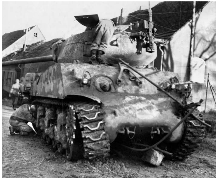
ABOVE: While one man looks into the turret of a Sherman, another mechanic (left) works to re-attach a track that has come off after the tank drove into a ditch in the Vosges region of France, December 1944. Maintenance personnel often had to retrieve the torn and burned bodies of crewmen from the tanks' interiors. OPPOSITE: Using a Federal C-2 wrecker, a maintenance crew installs a new radial airplane engine in a 2nd Armored Division Sherman tank named "Hurricane" near the front lines at Le Teilleul, France, east of Avranches, July 1944.
