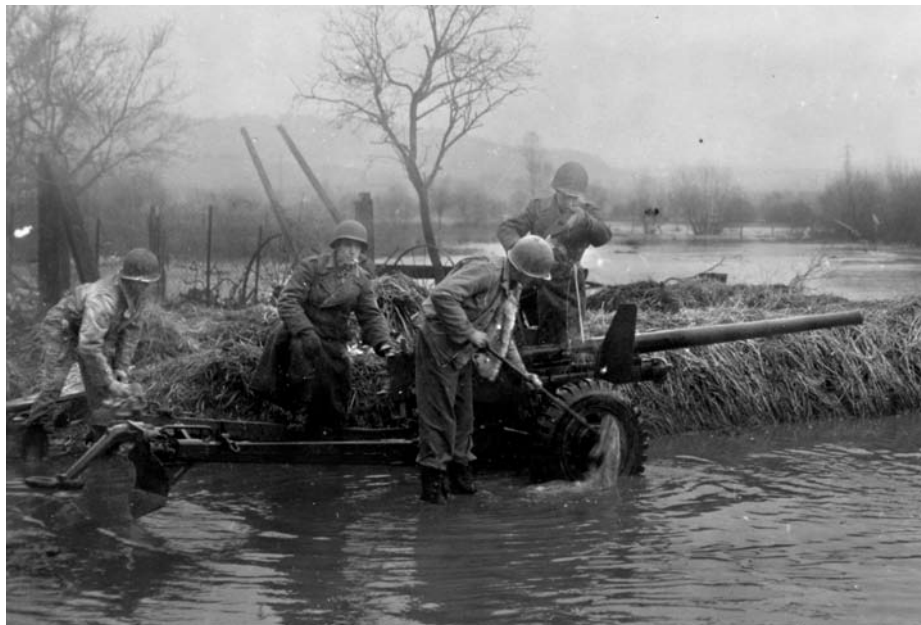
Gun crewmen use the Moselle River to wash the mud off their 57mm antitank weapon. The gun had a muzzle velocity of about 3,000 feet per minute and the antitank round could penetrate two inches of armor plate at 100 yards, but was virtually useless against the thicker frontal armor found on most panzers.
