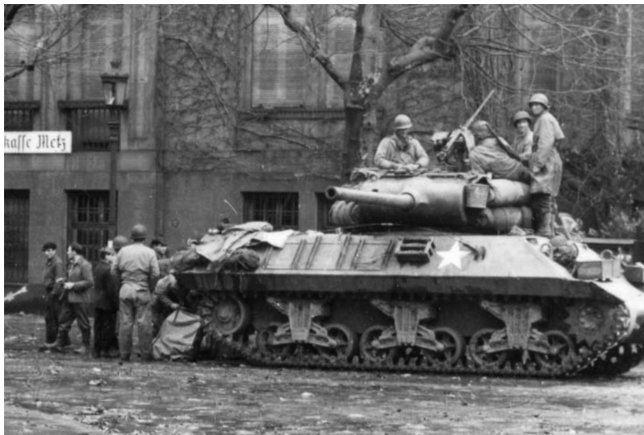
French civilians (left) receive provisions from members of a tank-destroyer unit in Metz, November 21, 1944. The M-10 tank destroyer pictured, built onto the same chassis used by M-4 Shermans, mounts a .50-caliber machine gun and a 3-inch main gun in its open-top turret.
