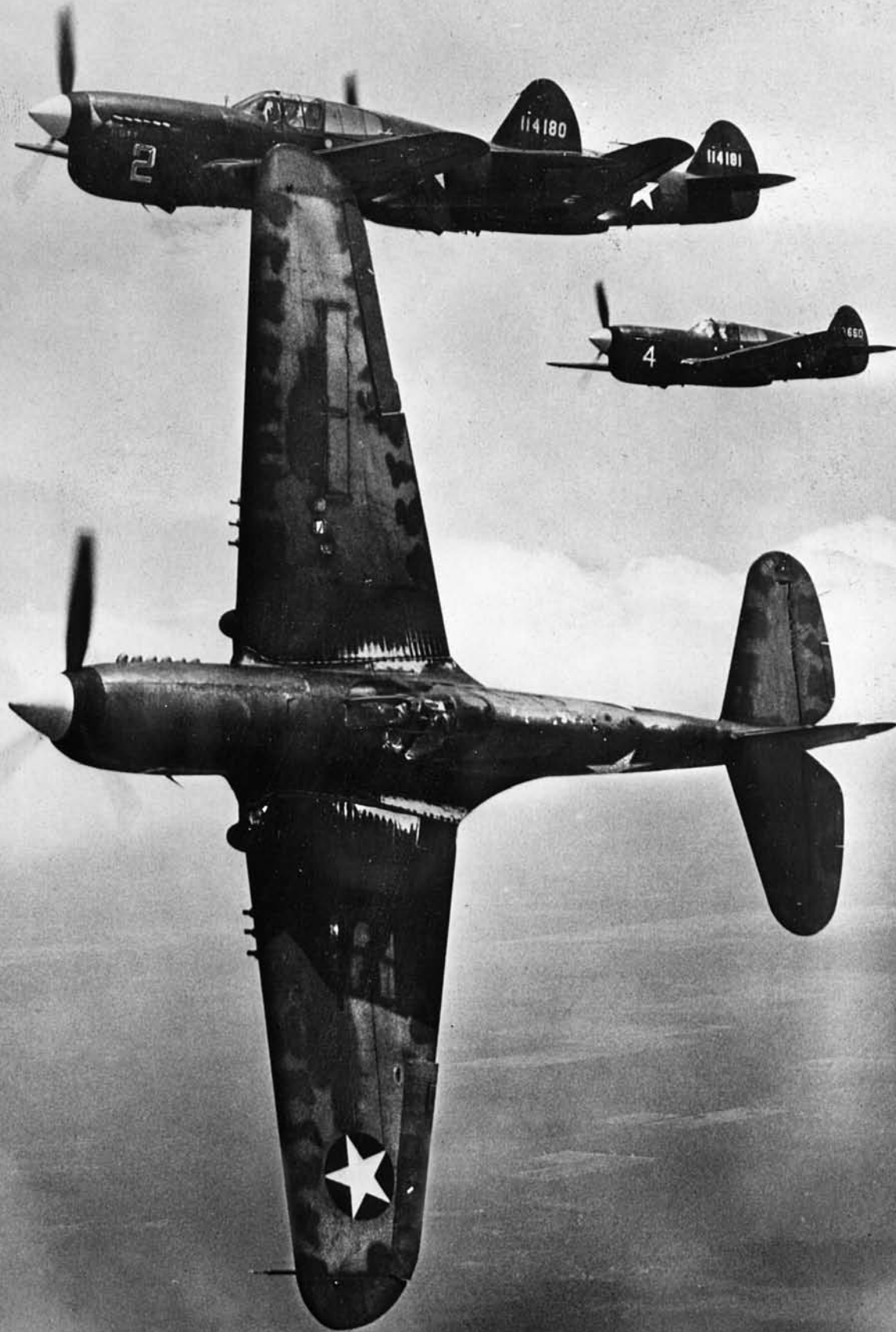
The sturdy Curtiss P-40 "Warhawks," shown here, with their liquid-cooled V-12 Allison engines, were outclassed by Japan's faster, more maneuverable Mitsubishi "Zero" fighter, but the American pilots made up for the P-40s shortcomings by being brave in the attack.
