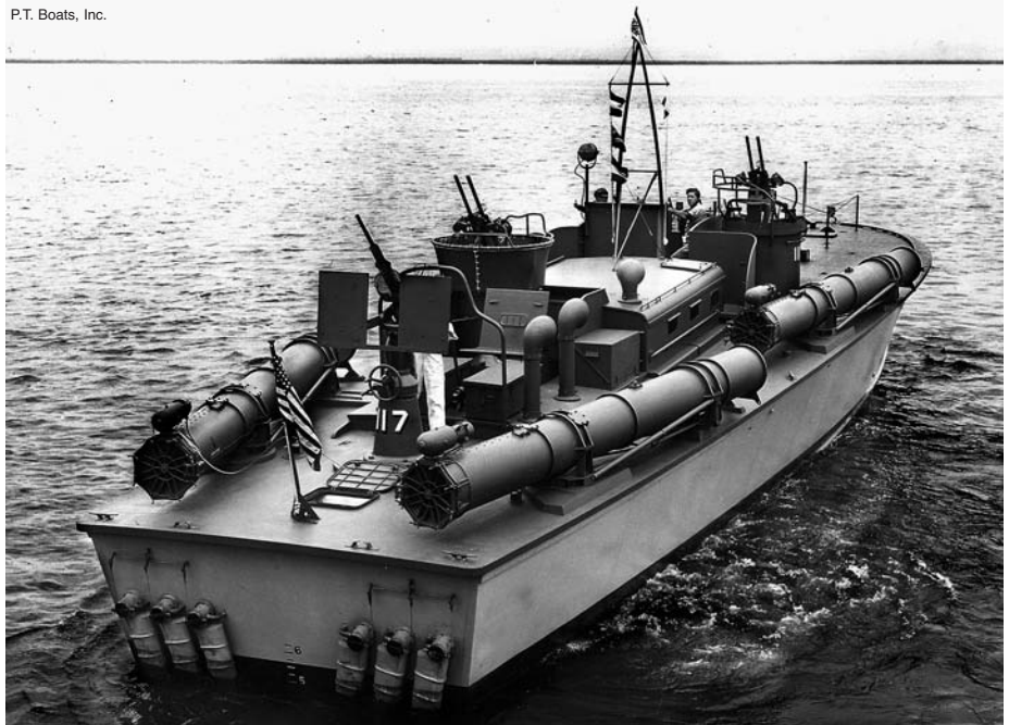
One of the small, fast motor torpedo patrol ("PT") boats made by Elco. The 80-foot-long boat carried up to four Mark 8 torpedos and could attain speeds between 25 and 27 knots.
