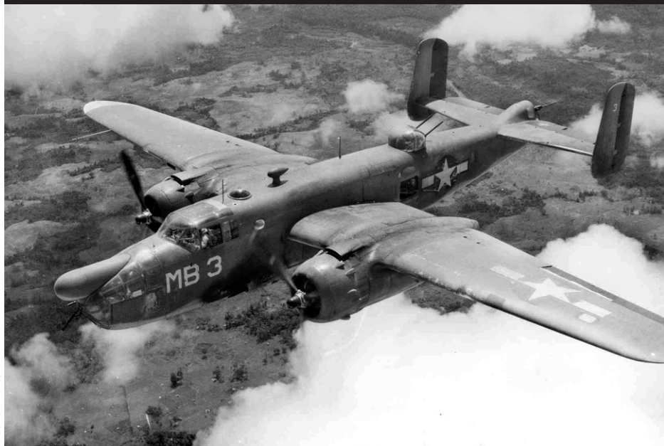
PBJ-1D Mitchell medium bomber assigned to a Philippines-based Marine Corps bombing squadron. The elongated "snout," commonly called a "hose nose," encompasses the sophisticated APS-3 search radar antenna. By 1943 eight VMB squadrons had been formed.
