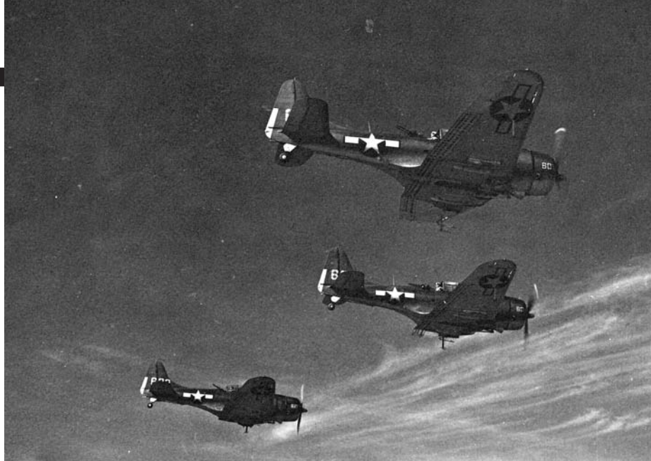
A trio of Dauntless SBDs patrols the skies. The aircraft, of which nearly 6,000 were built, was slower than its Japanese counterpart, the Aichi D3A2 "Val," but was steady in a dive and more resistant to battle damage.
