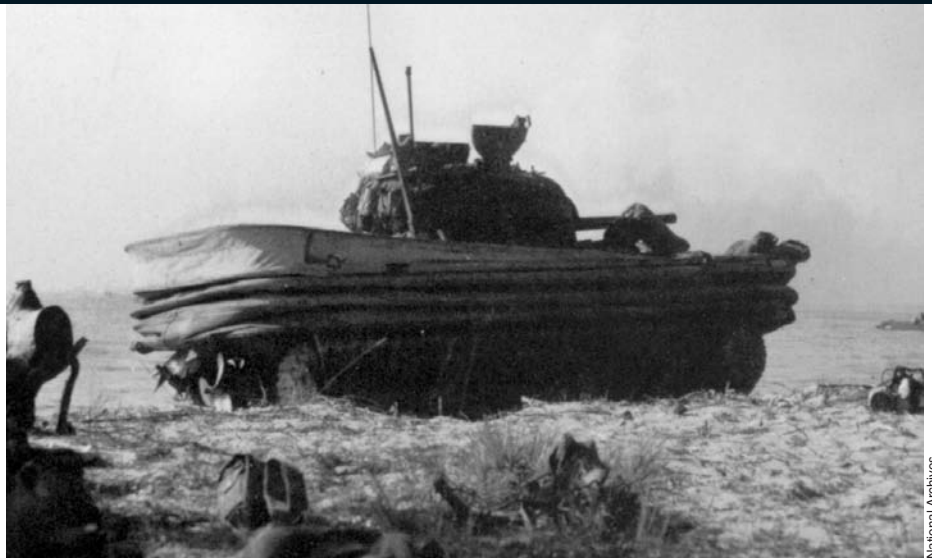
ABOVE: In theory, Hobart's Duplex Drive Sherman tanks, fitted with an inflatable canvas skirt, were supposed to be able to swim short distances, but rough seas at Normandy caused many of them to sink, drowning their crews. OPPOSITE: An M4 Sherman "Flail" or "Crab" tank fitted with a rotating drum and chains that pounded the ground ahead of the vehicle to detonate land mines.
