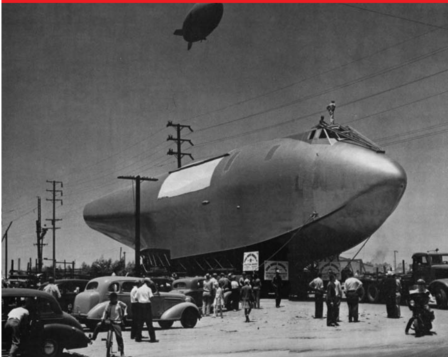
ABOVE: The wooden fuselage of the H-4 under construction. Innovative materials, including a new type of glue, had to be developed for the project, which cost more than $18 million. BELOW: Power lines needed to be removed for the fuselage's 28-mile journey in June 1946 from the Hughes Aircraft Company factory in Culver City to Pier E in Long Beach for final assembly. A blimp overhead follows the progress.
