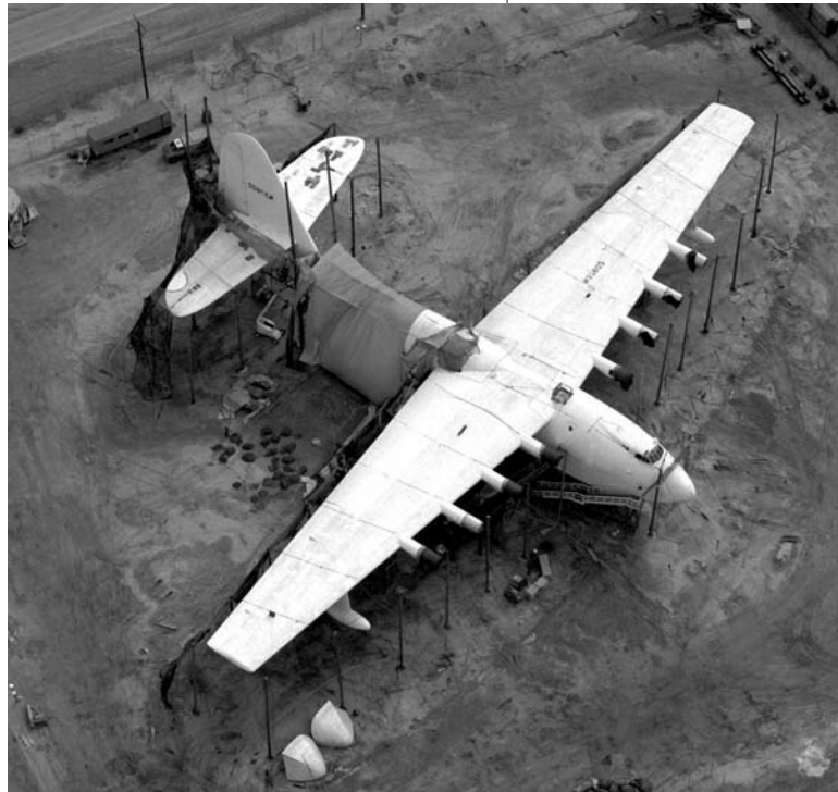
ABOVE: An aerial view of the H-4 Hercules shows its impressive size. The plane was almost 219 feet long from nose to tail and had a wingspan of 320 feet. BELOW: The tail of the H-4 was 85 feet—over five stories—high. The tail was deemed unstable after the initial flight according to some accounts.
