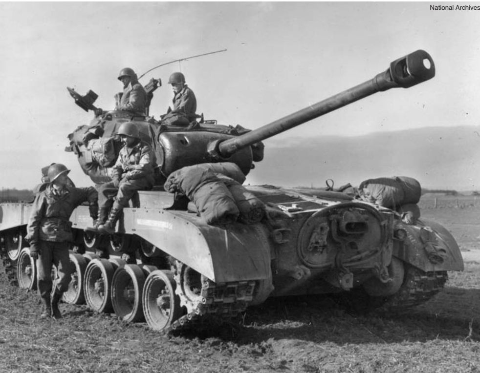
In March 1945, the crew of an American M26 Pershing heavy tank takes a break somewhere in western Germany. The Pershing, with its 90mm main gun, was developed as a match for the heavy German Tiger tank. While few of them reached the battlefields of Western Europe before the end of the war, a platoon of M26 Pershings from the 14th Tank Battalion fought at Remagen.
