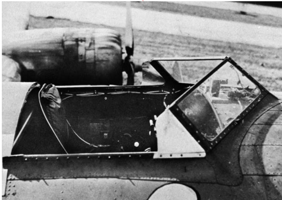
ABOVE: Standard Boeing B-17 Flying Fortress or Consolidated B-24 Liberator bombers were modified to participate in Operation Aphrodite. Here, the open cockpit of a modified bomber is shown with its top removed. BELOW: After antiaircraft fire has pushed it off course, an Operation Aphrodite drone crashes into the water short of its target. Operation Aphrodite was innovative and ahead of its time, but plagued with technical flaws.
