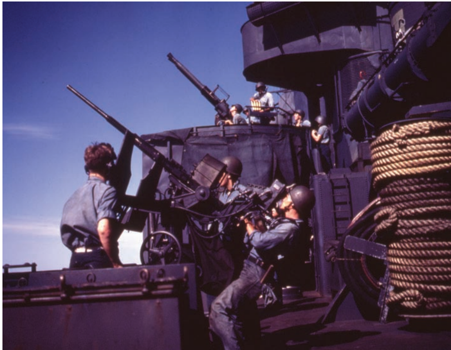
Destroyers bristled with guns for self-protection. This view shows a 20mm gun (foreground) and a Bofors 40mm gun behind it.
