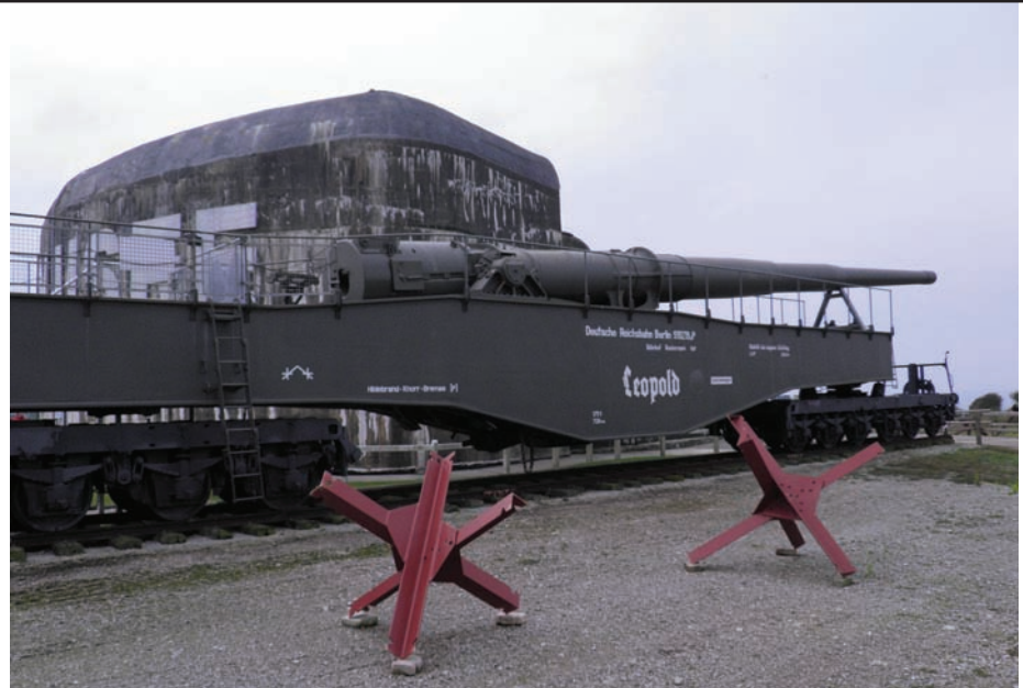
A Krupp M-5 280mm railway gun named “Leopold” stands outside the Batterie Todt casemate. The 70-foot-long barrel was capable of throwing a 562-pound shell 40 miles. At one time the Germans had 13-inch railroad guns along the coast.
