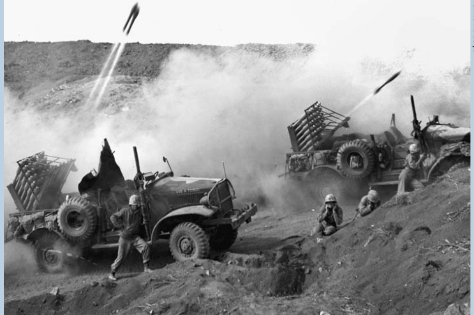
ABOVE: Marine rocketeers launch 4.5-inch projectiles toward Japanese emplacements on Iwo. The rocket units, being mobile, resorted to hit-and-run tactics to escape enemy counterfire. LEFT: Marines fire their water-cooled, .30-caliber machine gun at the enemy at the foot of Mount Suribachi on L + 3. OPPOSITE: Artillerymen of the 4th Marine Division use a 105mm howitzer to blast Japanese positions.
