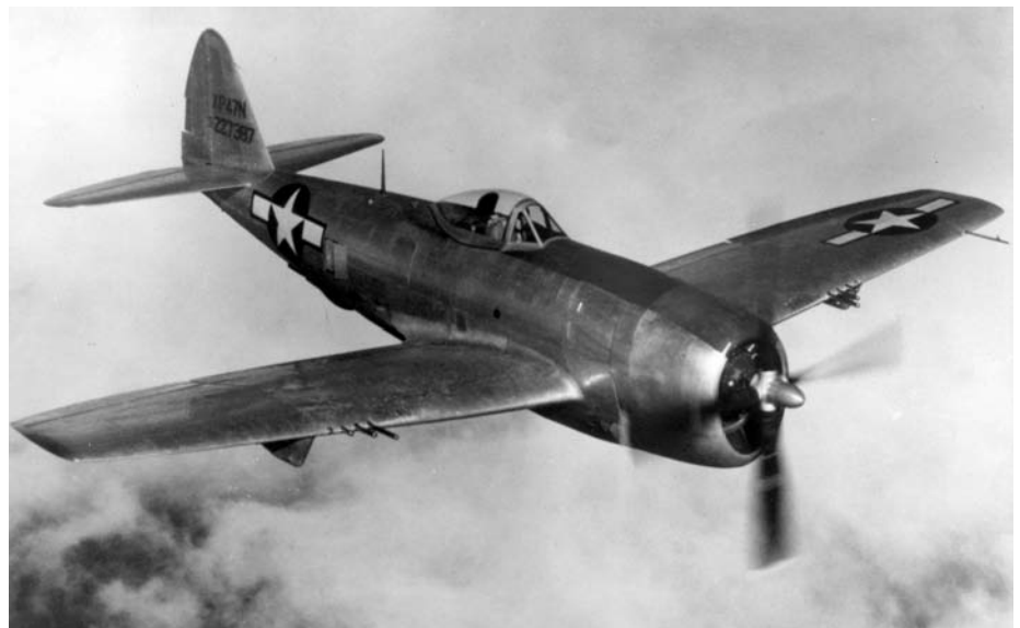
ABOVE: Used as both a high-altitude escort fighter and a low-level fighter-bomber, the P-47 quickly gained a reputation for ruggedness. Its sturdy construction and air-cooled radial engine enabled the Thunderbolt to absorb severe battle damage and keep flying. TOP: An unidentified pilot stands in front of a PT-19, one of the most popular primary trainers of the war, and the type which Ed Cottrell flew at Visalia, California. OPPOSITE: With machine guns blazing, a P-47 takes part in night gunnery practice. Ed Cottrell took his P-47 training at Wendover Field, Utah.
