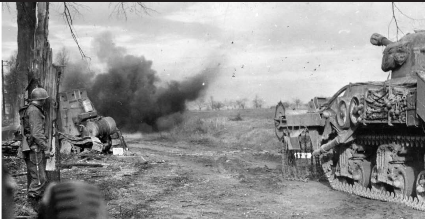
A GI from the 334th Regiment takes cover (left) as a Teller mine is detonated by engineers. A British-operated M4 Sherman tank with an anti-mine flail attached to its front waits before proceeding.
