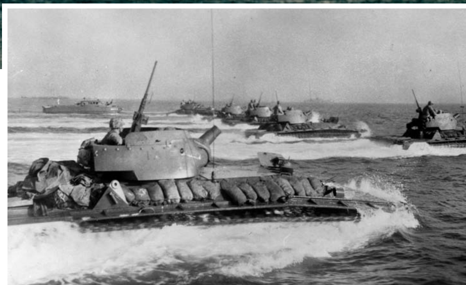
ABOVE: A line of Marine LVTs (Landing Vehicle Tracked) with their short-barrelled howitzers and cargo of Marines plunges through the surf on the way to their assigned beachhead. TOP: A panoramic color photo showing scores of landing craft and LTVs during Operation Iceberg—the invasion of Okinawa on L-Day, April 1, 1945.
