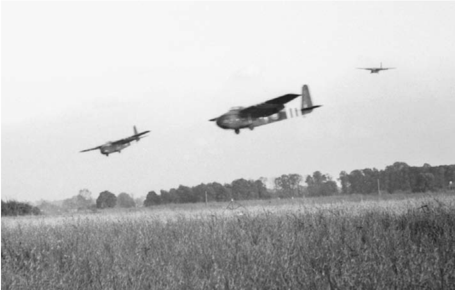
Hamilcar gliders of the British 6th Airborne Division land near the town of Ranville, France, on June 6, 1944. These gliders are carrying Tetrarch light tanks to support the offensive operations of the airborne troops.
