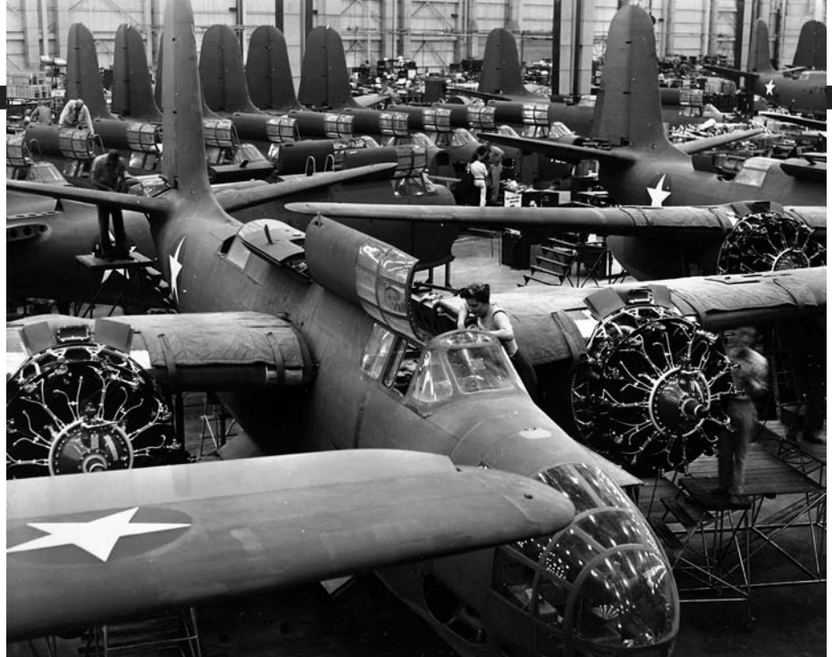
A-20 Havocs are assembled at one of the Douglas Aircraft's California factories. Most plants worked round the clock, seven days a week.
