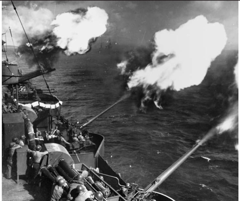
ABOVE: Five-inch guns of the cruiser USS Wichita soften up Japanese targets on Saipan, June 13, 1944. The guns' simultaneous discharge indicates they are firing under director control. BELOW: LVTs (Landing Vehicle, Tracked) known as "Buffalos" carry Marines through the surf on the way to a Saipan beachhead, June 15, 1944.
