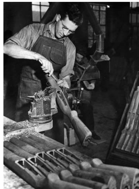
ABOVE: A worker finishes the wooden stock for an M1 Garand. More than 400,000 M1s were produced in the U.S. during World War II, at the rate of 1,000 a day. BELOW: John C. Garand, an inventor and engineer with the Springfield Arsenal, poses with the rifle that bears his name. OPPOSITE: A young soldier of the armored forces trains with a Springfield Arsenal .30-06 M1 Garand rifle at Fort Knox, Kentucky, in early 1942. Soldiers liked the rifle’s rugged construction and dependable operation. A skilled marksman could hit targets at a range of 450-500 yards.
