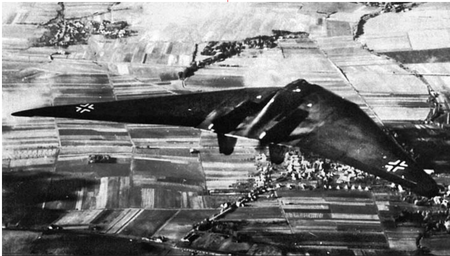
ABOVE: The exotic (and ultimately impractical) jet-powered Horten Ho-229 “flying wing” bomber takes a test flight over Germany, 1943. BELOW: Two U.S. Air Force airmen pose in front of an Ho-229 that was captured by the Americans at the end of the war.
