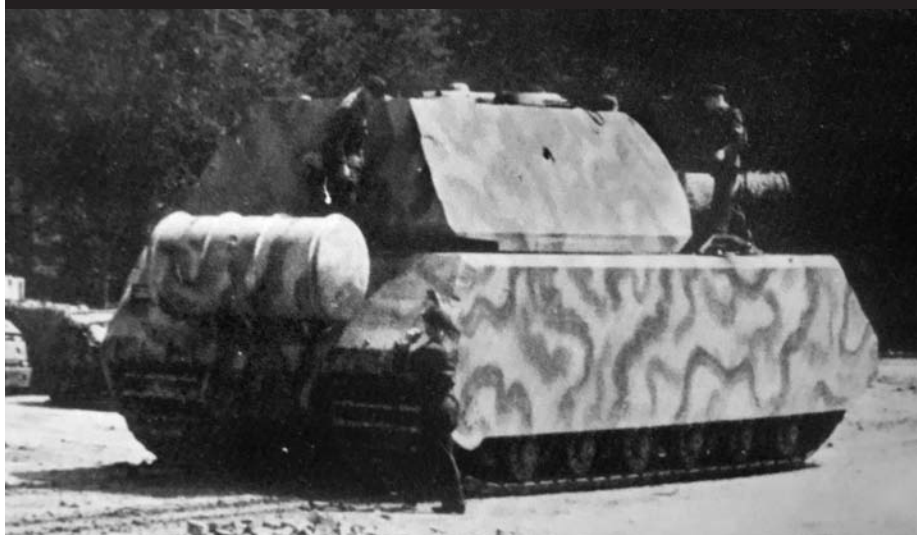
ABOVE: Porsche's 68-ton "Elefant" tank destroyer, with 88mm gun, was powerful but mechanically unreliable. BELOW: The Panzer VIII "Maus" weighed in at 188 tons but never made it to the battlefield; the two prototypes were captured by the Soviets.
