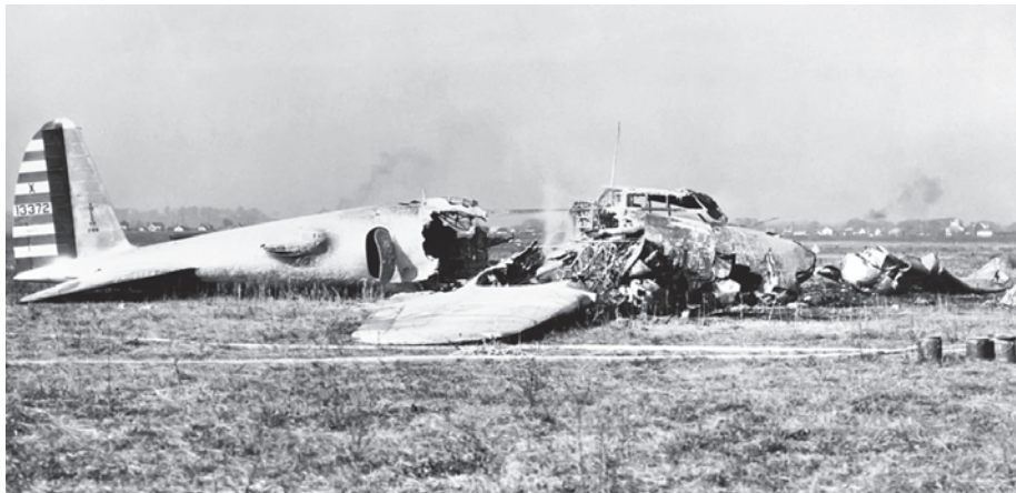
Before and After: Boeing XB-17, Model 299, the prototype for the B-17, crashed at Wright Field, Ohio, on October 30, 1935, killing the pilot and co-pilot due to a ground crewman's error. Despite the accident, the government awarded Boeing a contract to start mass producing the "Flying Fortress." INSET: The doomed passengers pose before a demonstration flight of a CG-4A glider in St. Louis, August 1, 1943. William Robertson, head of the company that built it, is pictured third from right.
