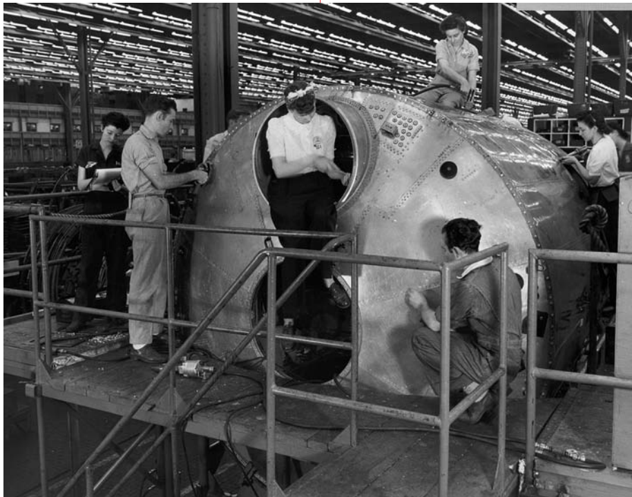
A crew of men and women work on the pressurized cockpit section of one of the big bombers in 1944. More than 600 of the 3,970 B-29s were produced at the Marietta factory which, now owned by Lockheed Martin, still produces aircraft for the U.S. Air Force.
