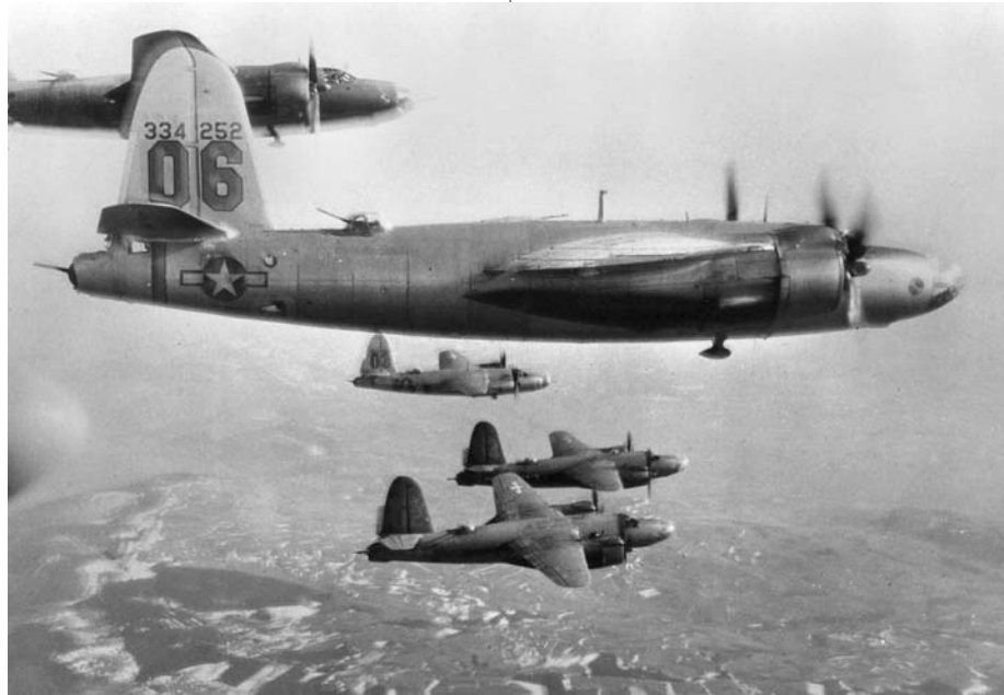
A formation of USAAF B-26 "Marauders" from the 320th Bomb Group, one of the units that took part in Operation Corkscrew. The B-26 could carry 4,000-5,000 pounds of ordnance.
