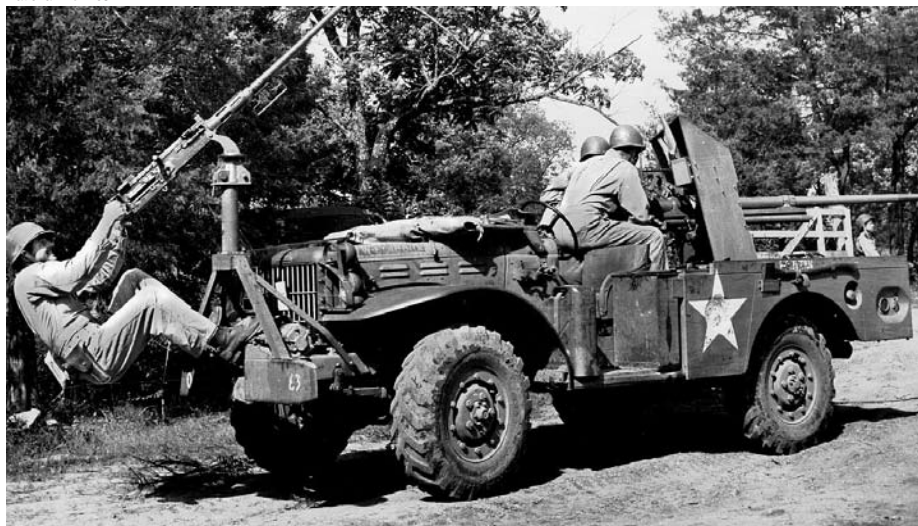
Shown on maneuvers in Tennessee in 1943, this M6 antitank vehicle is armed with a 37mm antitank gun mounted in the bed and a .50-caliber machine gun for antipersonnel or anti-aircraft use.
