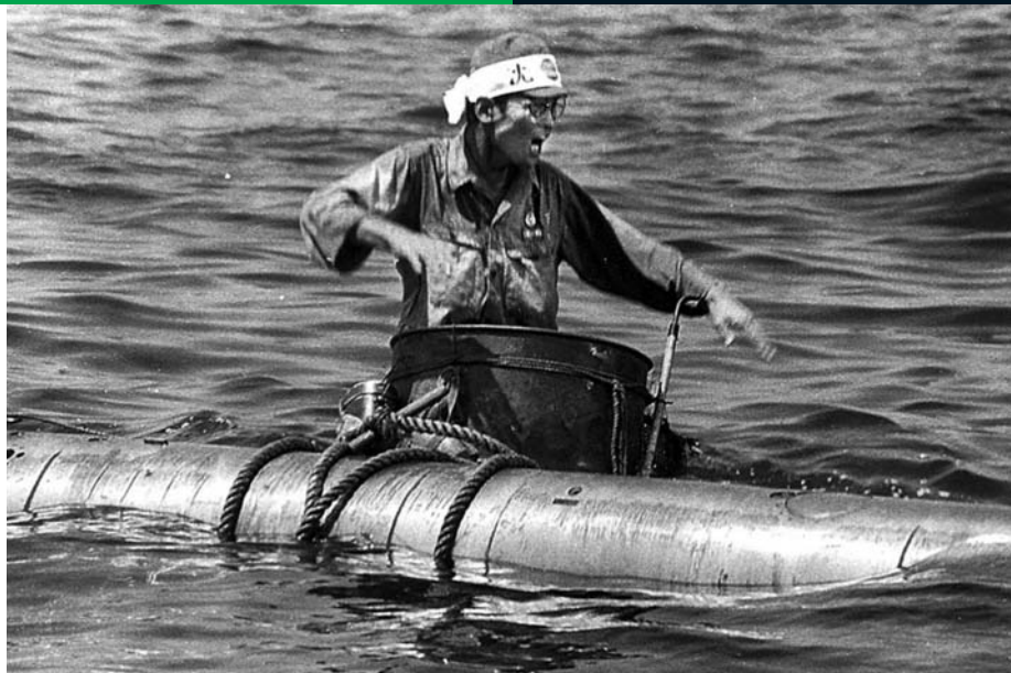
A Japanese Kaiten pilot in training maneuvers. The one-man subs were made from Japan's successful Type 93 torpedo.
