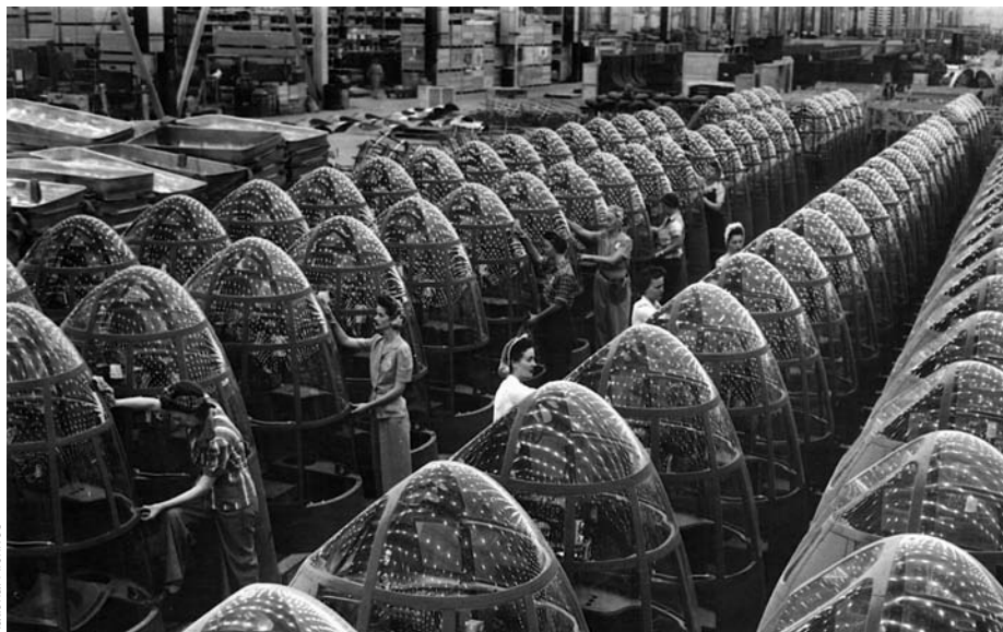
Female workers finish transparent noses built for A-20 attack bombers at Douglas Aircraft's Long Beach, Calif. manufacturing facility. The Japanese high command severely underestimated the Allied industrial capabilities, with disastrous results.
