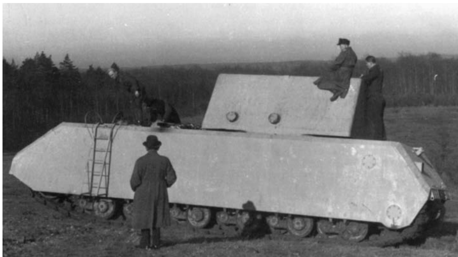
ABOVE: The prototype has a weight in place of the 50 ton turret. BELOW: Weighing over 100 tons, the Maus was ungainly on the battlefield and proved to be prone to mechanical failure.
