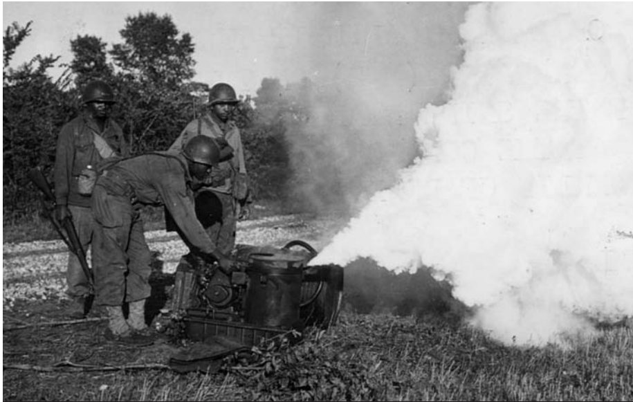
Testing an M-2 smoke generator along the banks of the Seine River in France, members of the 161st Chemical Company produce a thick pall of oily concealment.
