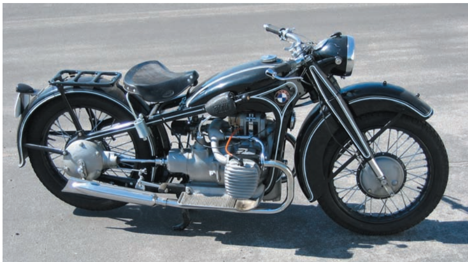
ABOVE: In 1935, BMW introduced its side-valve R16 which, along with the overhead-valve R17, was the world's first production motorcycle using a telescopic fork. OPPOSITE: Taking a nap along a dusty roadside, a motorcyclist tries to get some rest during the German advance across Russia.
