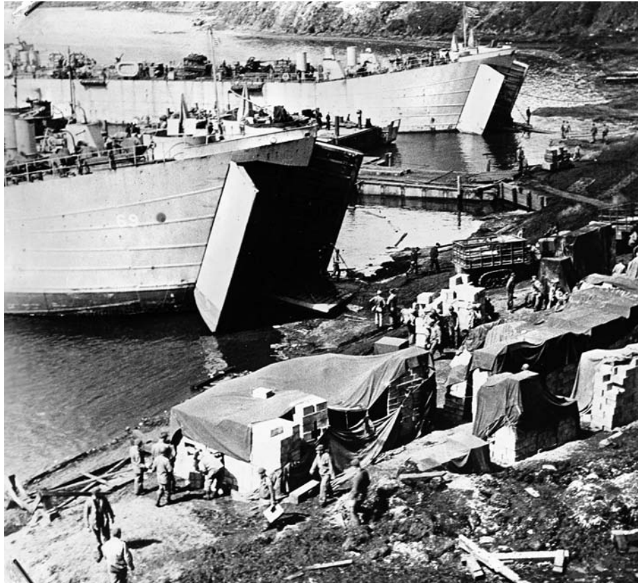
Coast Guardsmen and soldiers of the U.S. Army unload equipment and supplies on a beach in support of Allied landings. Note the large swinging doors of the LSTs (Landing Ship, Tank), which allowed the vessels to transport heavy loads, including tanks and other armored vehicles.
