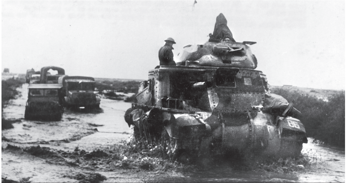
During fighting in North Africa, British troops ride through heavy rain and mud across the Libyan landscape. Their Grant tank mounts a 37mm gun in a small turret and a sponson mounted 75mm gun.
