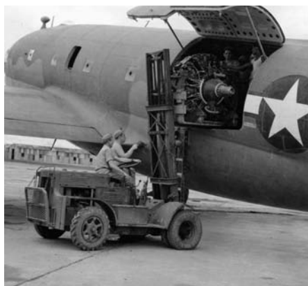
A replacement engine for a Boeing B-29 heavy bomber arrives in China aboard a C-46 transport. B-29 engines and replacement parts were a priority for Hump flights during the effort to mount a bombing campaign against Japan from airfields in China. (National Archives)
