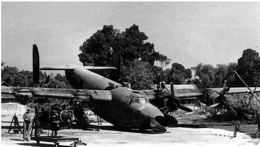
BELOW: A C-87 transport, which has crashed at an airfield in India, is salvaged by ground crewmen in the hopes that it will be airworthy once again. The C-87 was the transport version of the B-24 Liberator heavy bomber. (Both: National Archives)
