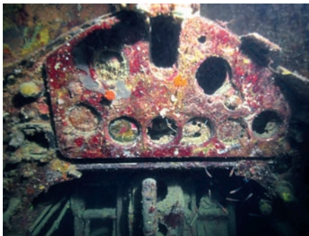
ABOVE: A pair of spadefish glide past the exposed empennage of the Gavutu Wildcat. LEFT: The instrument panel of the Gavutu Wildcat. Years of corrosion have caused some instruments to dislodge from the panel and fall behind it.
