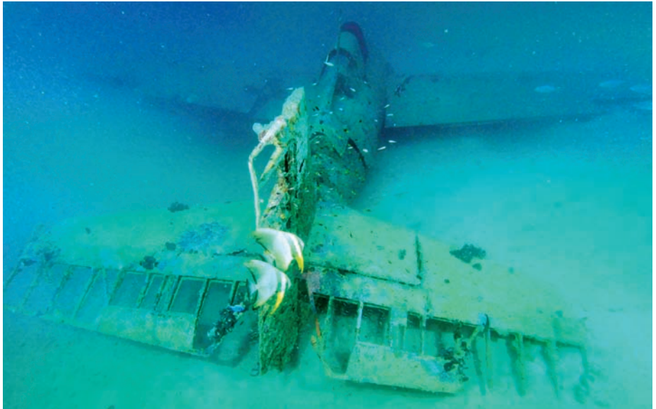
ABOVE: A pair of spadefish glide past the exposed empennage of the Gavutu Wildcat. LEFT: The instrument panel of the Gavutu Wildcat. Years of corrosion have caused some instruments to dislodge from the panel and fall behind it.
