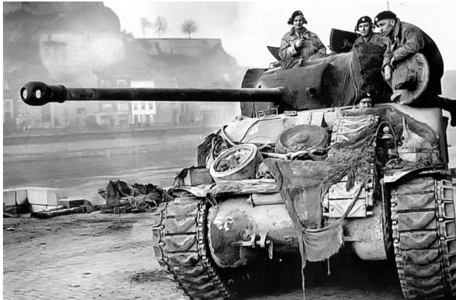
ABOVE: Crewmen pause in the chassis and turret of a Sherman Firefly tank of the British Coldstream Guards during the ground advance into the Netherlands. Six Fireflies, modified from the original Sherman configuration to carry a 17-pounder gun and belonging to the 1st Battalion, Coldstream Guards helped Company B, 505th Parachute Infantry Regiment repulse a German attack on the Heumen Bridge. TOP: German paratroopers of the 5th Fallschirmjäger Division fire a captured American-made Browning M1919 A4 .30-caliber machine gun during the fighting in Operation Market-Garden. OPPOSITE: Two camouflaged German armored vehicles on a road in the Netherlands during Market-Garden. These are the Flakpanzer IV Möbelwagen, armed with a 37mm anti-aircraft gun. A variant of the PzKpfw. IV medium tank, the Flakpanzer IV, or similar armored vehicles, may be what troopers of the 82nd reported as PzKpfw. V “Panthers.”
