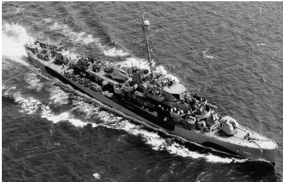
ABOVE: Shown under way off Long Island in August 1944, the destroyer escort USS Kendall E. Campbell was a John C. Butler-class ship, the fastest class of the vessel built. These small, versatile warships were powered by geared steam turbines. The Kendall E. Campbell is painted in a measure 32 camouflage scheme, and its 5-inch gun mounts are enclosed. RIGHT: This photograph of the stern of the destroyer escort USS Menges shows the 21-inch torpedo battery that originally equipped such warships starting with the Buckley class. Also note the 20mm and 40mm antiaircraft mounts, the 3-inch deck gun, depth charge throwers, and racks. (Both: National Archives)
