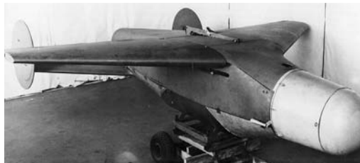
The ASM-N-2 BAT (SWOD Mk 9) was a glide bomb constructed of steel and wood which carried a warhead fashioned from a 1,000-pound general purpose bomb.
