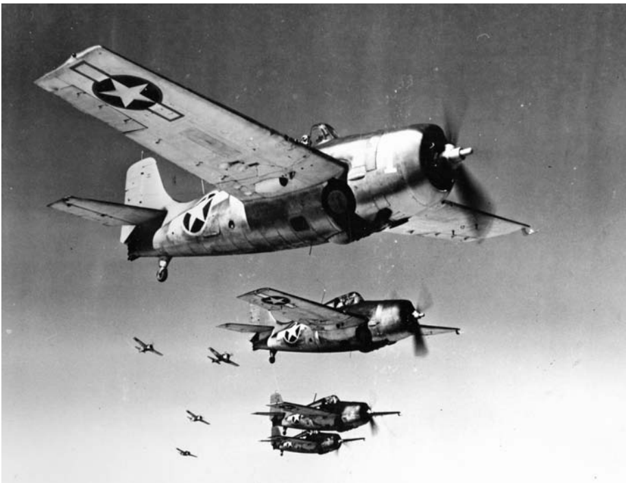
ABOVE: Wildcat fighters fly in formation in the South Pacific on September 22, 1943. Although the Grumman F4F was not as nimble as its Japanese Zero adversary, it was well armored and packed a heavy punch with .50-caliber machine guns. TOP: Taxiing on the runway at Henderson Field on Guadalcanal, this Grumman F4F Wildcat fighter has just landed after arriving from an aircraft carrier. The external fuel tank attached to the right wing extended the fighter's range.
