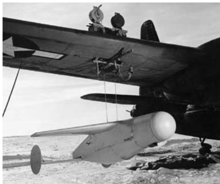
A BAT missile is lifted into position on a PB4Y aircraft prior to a mission in the Pacific. The BAT was actually tested in combat as the war against Japan neared its close.
