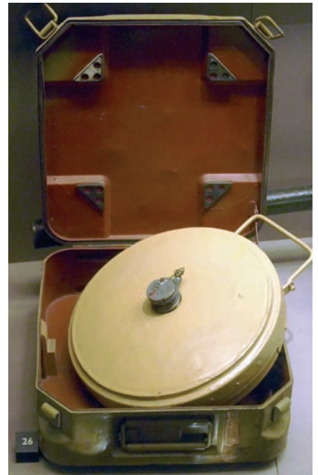
ABOVE: Literally millions of mines were sown by the warring armies during the fighting in Europe. Here, German soldiers place antitank mines near defensive positions on the Eastern Front in 1944. RIGHT TOP: A German Tellermine, used against enemy tanks and armored vehicles, is shown in its carrying case. CENTER: An American paratrooper locates an antipersonnel S-mine 35 with an S.Mi.Z.35 pressure fuse. BOTTOM: The small but powerful antipersonnel Schü-mine 42 belies its sinister capability to disable the unfortunate soldier who stepped on the device, which was encased in wood and difficult to detect.
