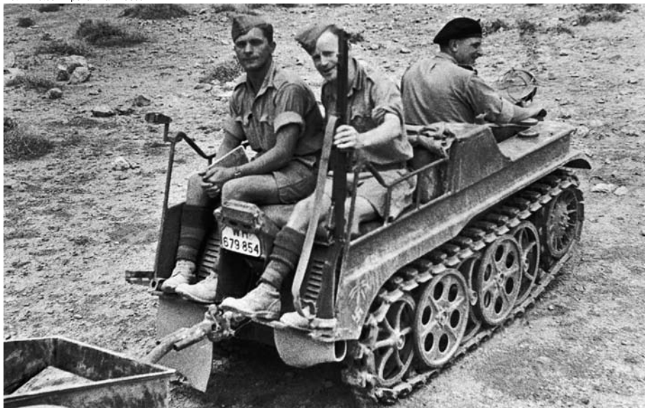
ABOVE: British soldiers take a ride on a captured Kettenkrad in June 1942. Although it appeared somewhat awkward, the machine proved durable and capable of traversing difficult terrain. TOP: Abandoned by retreating German troops, this Kettenkrad is inspected by a British soldier in North Africa. The Kettenkrad was a curious blend of motorcycle and tracked troop carrier.
