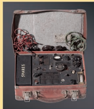
A WWII spy radio "Type A MK.III" of the British Special Operation Executive (SOE)
