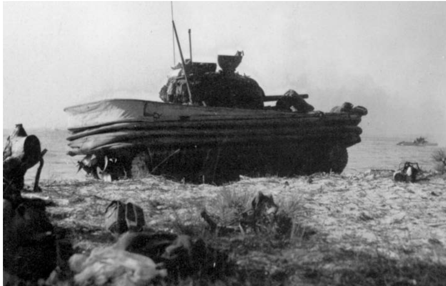
The DD (Duplex Drive) Sherman tank was fitted with a specially designed canvas screen for flotation, which theoretically would allow the tank to navigate short stretches of water. When the screen was lowered, the Sherman's 75mm cannon could be put into action.
