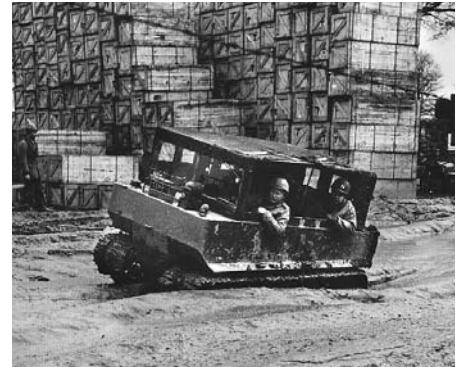
Geoffrey Pyke designed the vehicle that became the U.S. M26 Weasel. Although it was intended for use in snow, it found application on the muddy roads of France.
