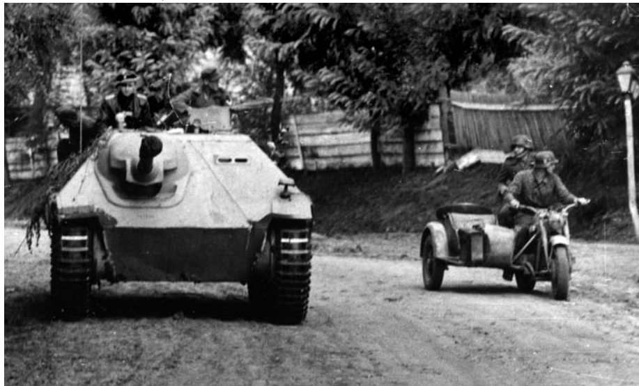
This Hetzer of the Waffen SS Division Florian Geyer was photographed in Hungary in 1944. The 75mm main gun of the Hetzer was capable of knocking out most Allied tanks fielded during the war.
