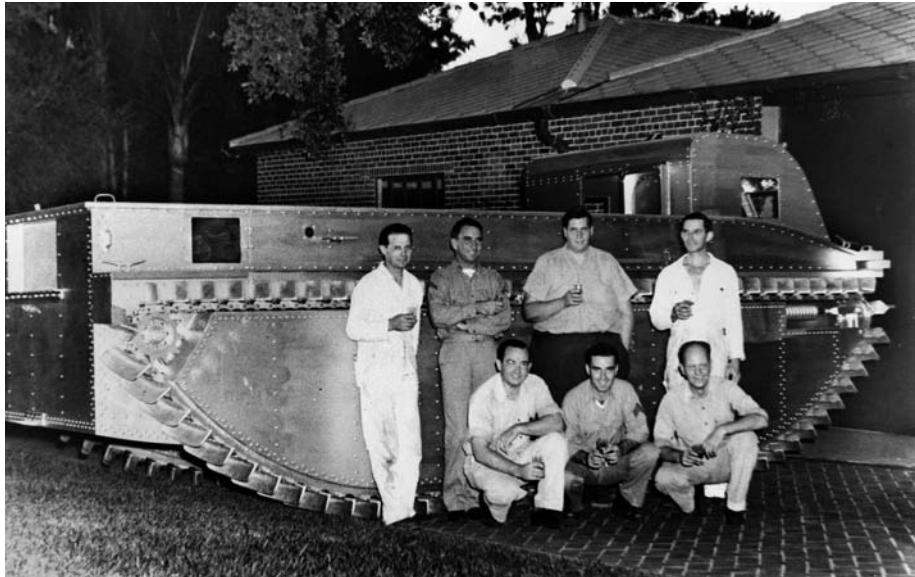
Photographed in the driveway of Donald Roebling's Florida estate, Roebling and his co-workers pose with the fourth generation amphibious vehicle that became the famed Amtrak during World War II.
