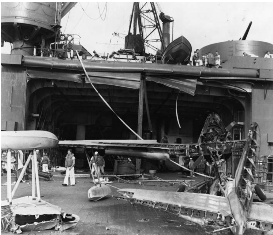
ABOVE: Smoke boils up from the USS Curtiss after the ship was struck by a crippled Japanese dive bomber during the attack on Pearl Harbor, December 7, 1941. BELOW: The Curtiss sustained extensive damage to its hangar when a Japanese bomb penetrated the boat deck and three lower decks and exploded in the magazine of the No. 4 gun. Eighteen men were killed, and the 5-inch weapon was put out of action.
