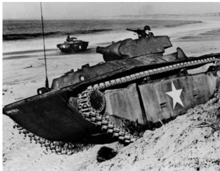
The military upgunned the LVT-4 to produce the LVT-4(A) mounting a 75mm howitzer. The howitzer was capable of taking on Japanese bunkers and pillboxes during island fighting.
