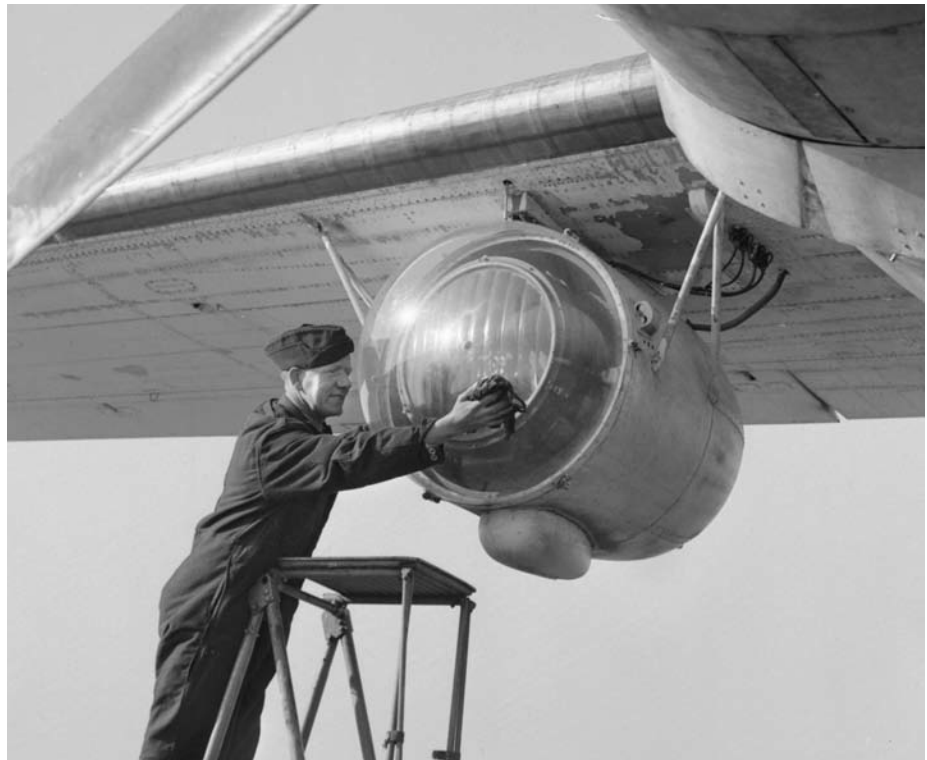
ABOVE: An excellent innovation deployed with sub-hunting aircraft that patrolled the Bay of Biscay, the Leigh Light was used to illuminate German U-boats on the surface and facilitate the speed of attacks. In this photo a Royal Air Force ground crewman cleans the plexiglass cover of a Leigh Light that has been installed under the wing of a Consolidated Liberator bomber. OPPOSITE: Royal Air Force armorers load 250-pound Mark VIII depth charges aboard a Consolidated Liberator Mark VA bomber of RAF Coastal Command. This aircraft is from No. 53 Squadron based at St. Eval.
