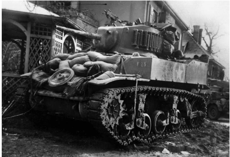
ABOVE: The Stuart light tank was a superb reconnaissance vehicle but its 37mm main weapon was useless against German armor. The 106th Cavalry Squadron fielded the Stuart until the spring of 1945, when medium tanks with 75mm guns became available. This photo was taken in Ludweiler, Germany. BELOW: On January 2, 1945, the day after the German Army launched Operation Nordwind, engineers of the 106th Cavalry Squadron prepare a roadblock to slow the enemy advance a half mile from the town of Ludweiler, Germany.
