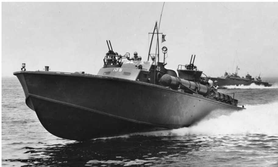
PT-105 is seen among a group of PT boats on maneuvers in the Atlantic shortly after completion in July 1942. The initial group of boats had no armament forward of the conn area, but the space was used later in the war for more firepower.
