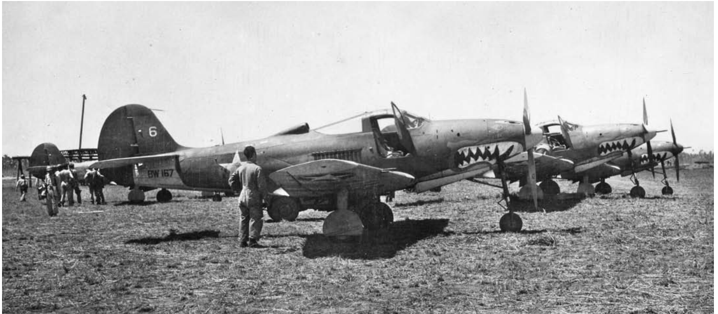
Photographed at Guadalcanal in October 1942, these Bell P-400 Airacobra fighter bombers are obviously battle worn. The Airacobra's cannon and machine gun armament proved well suited to reducing ground targets.
