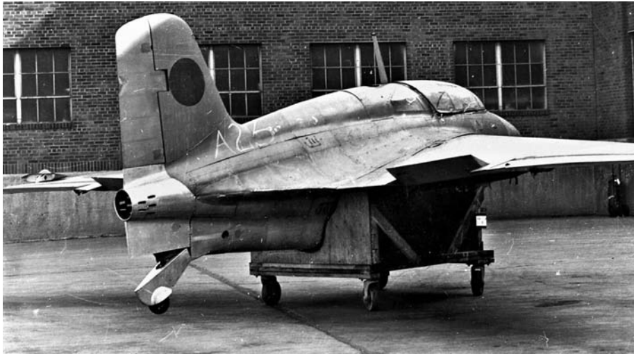
The Germans provided detailed plans of the Komet to their Japanese allies in the last days of World War II, and the Japanese constructed their own version of the rocket-powered interceptor, the Mitsubishi J8M1 Shusui.
