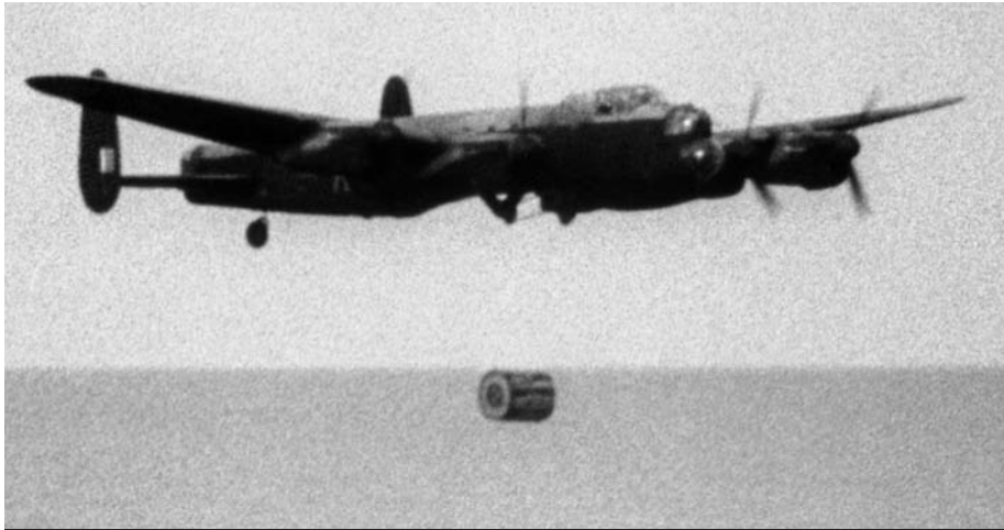
ABOVE: This Avro Lancaster heavy bomber of No. 617 Squadron RAF engages in training for Operation Chastise. During its training run, the bomber drops the Upkeep weapon on the bombing range at Reculver, Kent. RIGHT: Checking instrument settings in the crew compartment of his Lancaster B Mk. III, a flight engineer prepares for a mission
