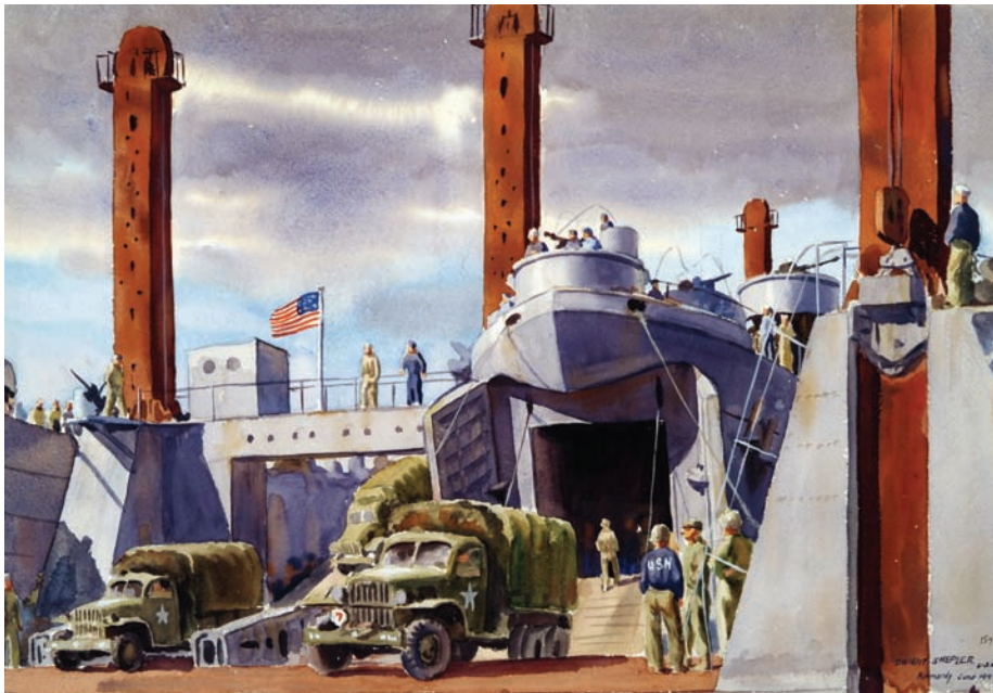
In this painting by artist Dwight Shepler, a Landing Ship, Tank (LST) discharges cargo from both its upper and lower decks onto a T-shaped formation of floating pier heads.
