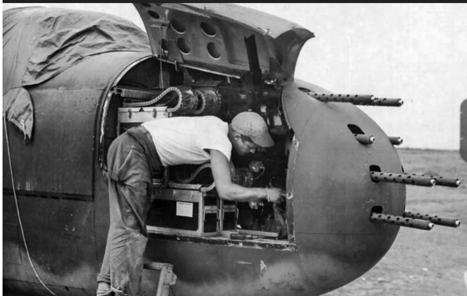
ABOVE: Workers assemble B-25 Mitchell medium bombers on the floor of the factory at North American Aviation in Kansas City, Kansas, in October 1942. BELOW: Some B-25s were modified as gunships to strafe enemy shipping or ground targets. In this photo, a ground crewman performs maintenance on one of eight .50-caliber machine guns packed into the plane's nose.
