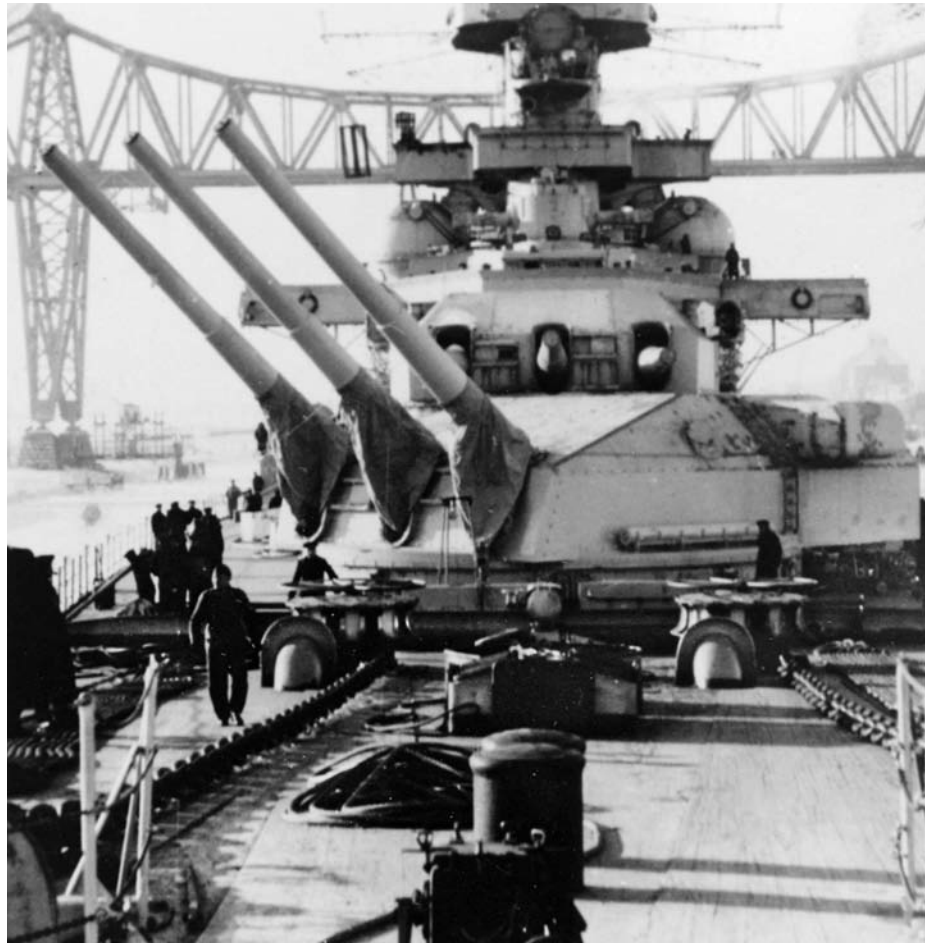
ABOVE: The two forward 11-inch main batteries of the battlecruiser Scharnhorst loom as the ship lies at anchor in the port of Kiel in the winter of 1940. Scharnhorst sank the British aircraft carrier HMS Glorious but was destroyed in the Battle of the North Cape. OPPOSITE: A large crowd gathered in June 1934 to watch the launching of the pocket battleship Graf Spee . Graf Spee came to grief in 1939, scuttled after the Battle of the River Plate.
