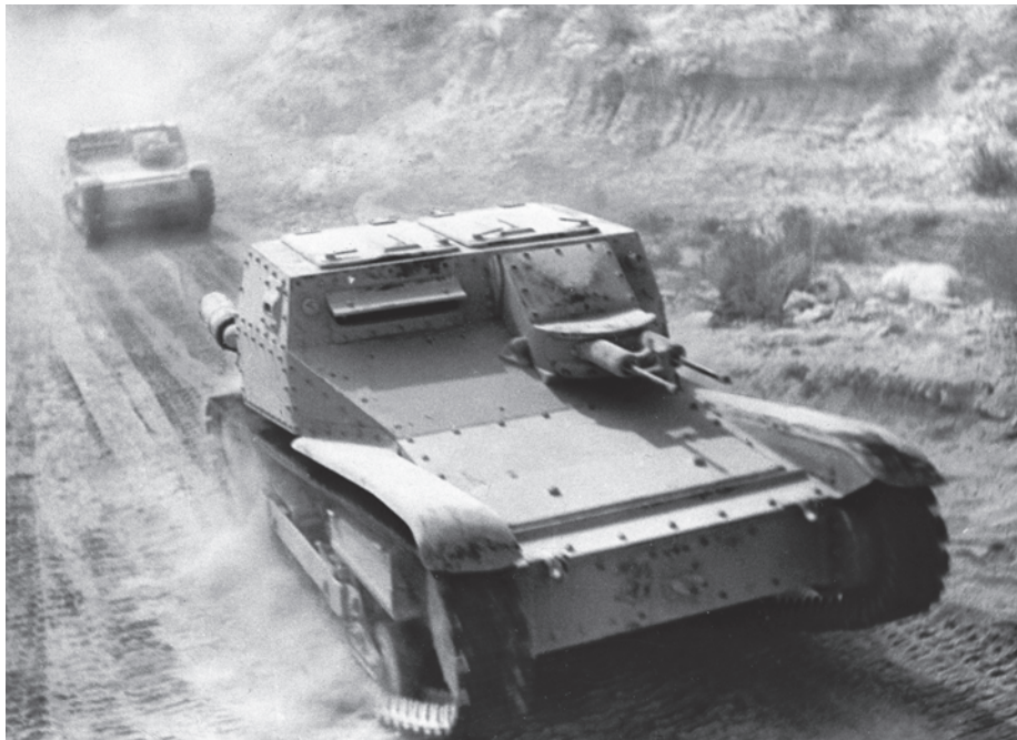
Early Italian tanks such as these L3/33 Carro Armato “fast tanks” were operated by two-man crews and armed only with machine guns.
