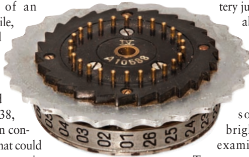
ABOVE: The German submarine U-505 was one of several captured on the high seas by U.S. Navy personnel, yielding codebooks that assisted in deciphering enemy communications. BELOW: A system of rotors was the key to the effectiveness of the German Enigma system.
