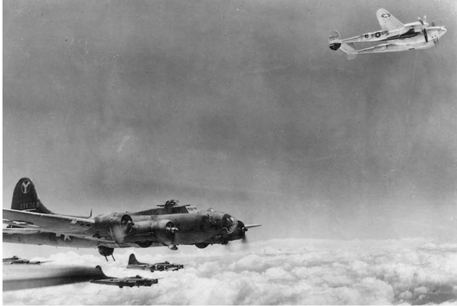
The Lockheed P-38 Lightning fighter, upper right, was a robust twin-boom and twin-engine aircraft that was capable of flying bomber escort missions and engaging in air-to-air combat. The Germans nicknamed the Lightning the "Fork-tailed Devil."
