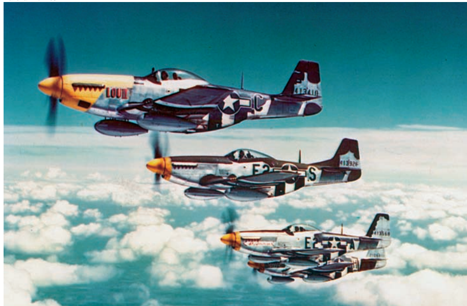
Carrying drop tanks to extend their range, a flight of P-51 Mustangs maintains formation in the skies over Europe. The P-51 became the premiere Allied long-range escort fighter of World War II, even reaching Berlin from airfields in England.
