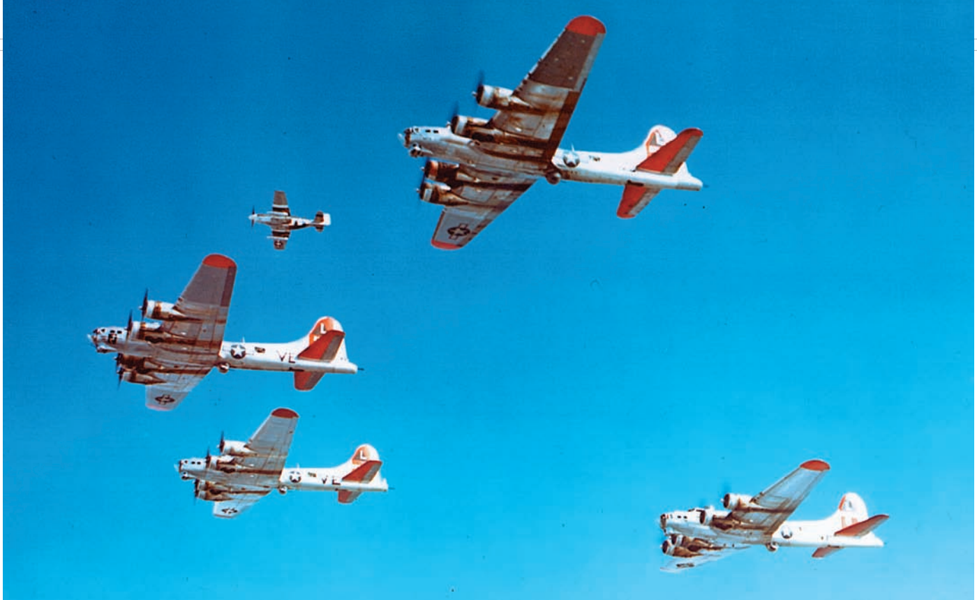
A P-51 Mustang fighter, upper left, flies escort duty with a formation of B-17 Flying Fortress bombers. The marriage of the North American airframe design and the Rolls-Royce Merlin engine produced a high-performance fighter that was originally conceived as a dive bomber powered by an Allison engine.
