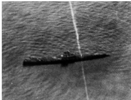
This photo was taken during the test of the Mark 14 torpedo off Newport, Rhode Island, on May 26, 1926. This torpedo, one of two fired, missed the targeted submarine hulk and failed to explode.
