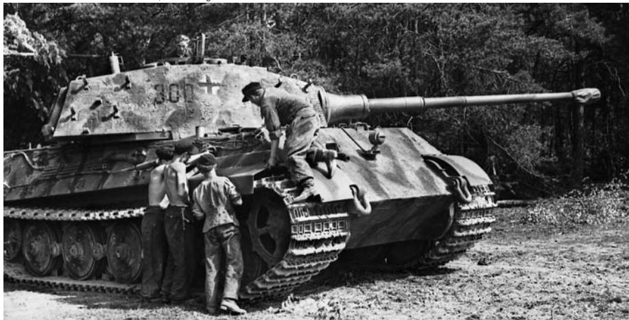
ABOVE: This PzKpfw. VI Tiger II sits at the edge of a French forest in June 1944, while crewmen appear to be changing the camouflage scheme. Although its 88mm high-velocity cannon was formidable, the tank was heavy, ponderously slow, and prone to mechanical failure in cross-country operations. BELOW: Engineers and dignitaries inspect the massive hulk of the Maus, an experimental tank of tremendous proportions. The concept of the Maus proved impractical, and only four prototypes were ever built.
