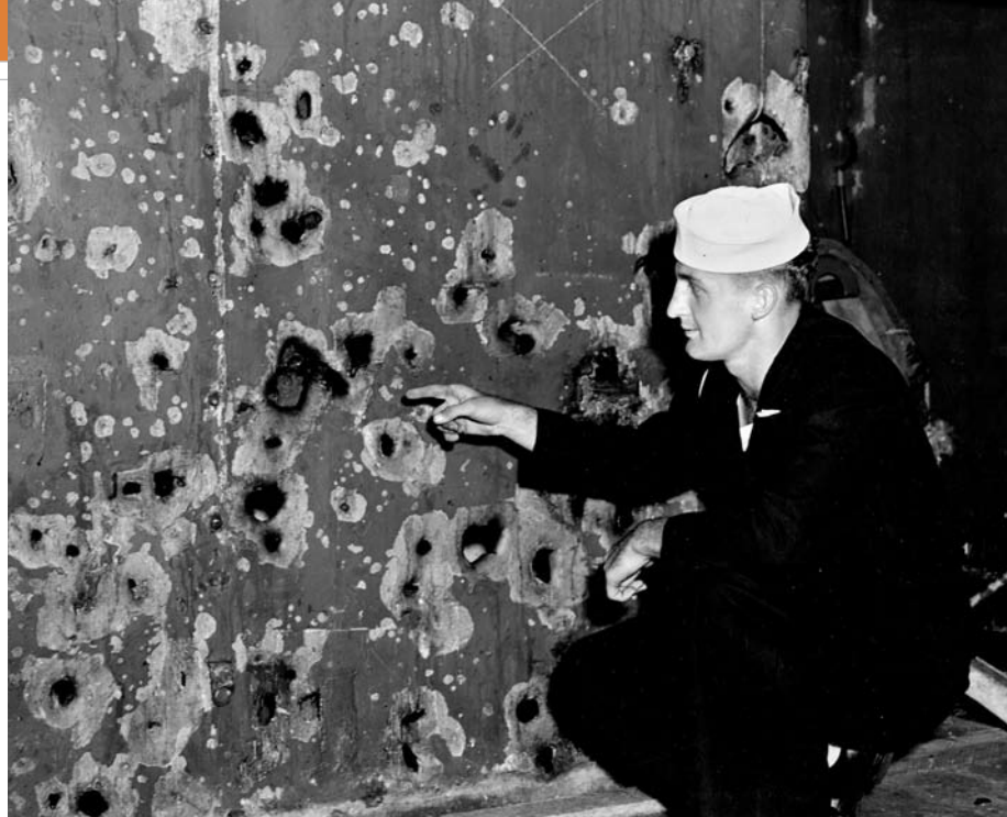
A sailor points to damage sustained by the cruiser USS Boise during the Battle of Cape Esperance. This shredded bulkhead was hit by fragments from a shell that exploded only 30 feet away. This photo was taken during repairs at the Philadelphia Navy Yard.
