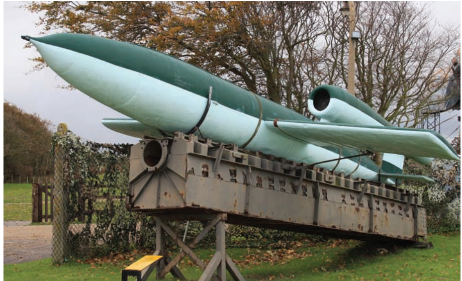
ABOVE: The V-1 flying bomb was powered by a pulse jet engine with just enough fuel to reach its destination. As the V-1 ran out of fuel, it plummeted indiscriminately to earth and exploded with devastating results. Many V-1s hit London and other British cities, causing civilian casualties. BELOW: A German V-2 rocket is raised into launching position at Cuxhaven in the Luneburg District of Lower Saxony.
