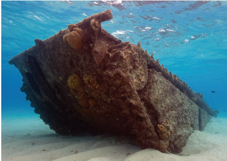
This LVT(A)-4 “Marianas Model” amphibious landing craft lies where it sank off the island of Saipan. The vehicle was capable of traversing coral reefs, delivering men and supplies to embattled beaches in the Pacific.
