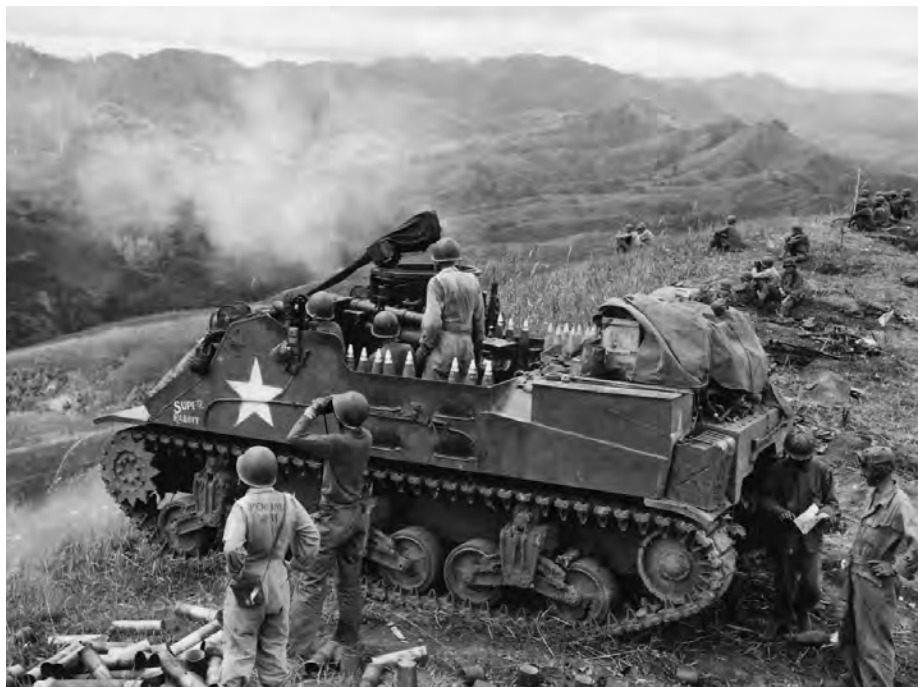
ABOVE: Members of the 40th ID man the “Super Rabbit,” a self-propelled M7 Priest armed with a 105-mm howitzer. The crew is firing at Japanese positions in the mountains of Luzon, Philippines, in February 1945. OPPOSITE: The 185th Infantry Regiment plants the American flag on top of Gusi Hill (Hill 1700) on February 25, 1945. The 40th ID took part in some of the fiercest fighting in the Philippines in the month-long fight for the Bamban Hills, a strategic area for the Imperial Japanese Navy as the headquarters for the 1st Combined Air Fleet.
