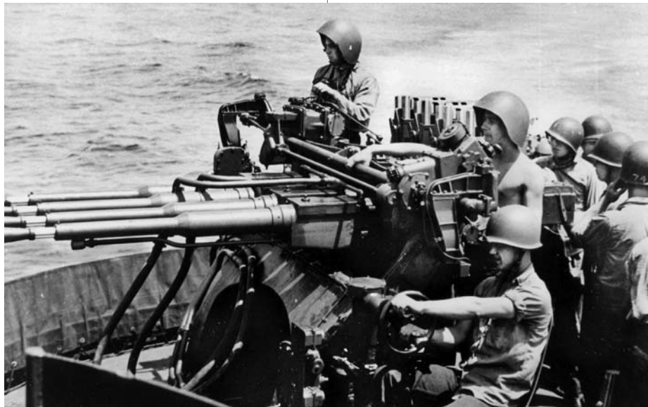
An anti-aircraft gun crew aboard the USS South Dakota services its 1.1-inch (.75-caliber) weapon during training. The 1.1-inch gun was prone to jam and proved unpopular with its crews during the Pacific War.
