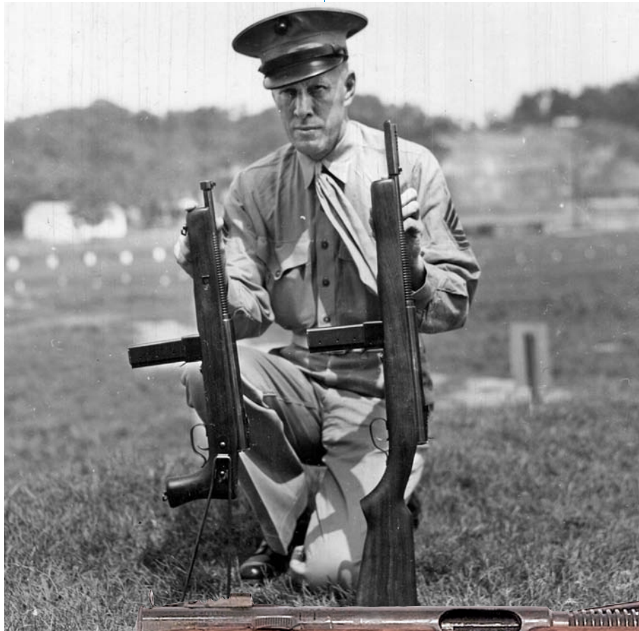
U.S. Marine Master Gunnery Sergeant V.J. Kavits poses with the Model 55 Reising submachine gun (left), with its pistol grip, folding wire stock, and shortened barrel, and the standard Model 50 Reising. Neither fulfilled the expectations of the U.S. Marine Corps.
